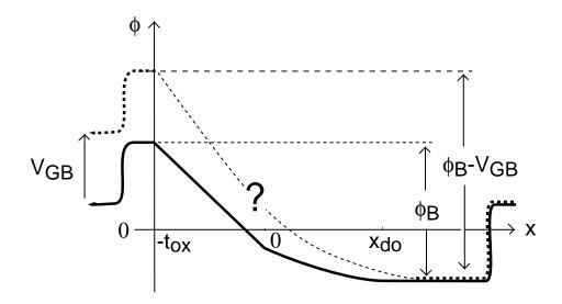
Oxide is insulator  $\Rightarrow$  no current anywhere in structure
