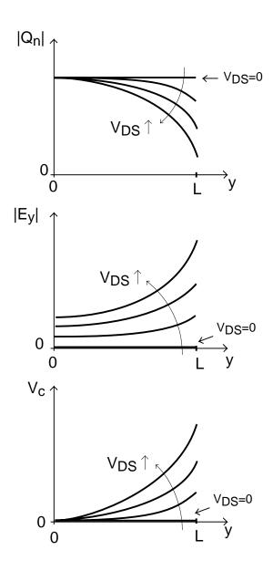
Ohmic drop along channel debiases inversion layer  $\Rightarrow$  current saturation
