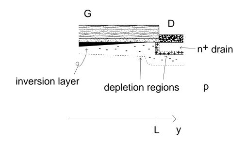
Voltage at pinch-off point (V = 0 at source):
