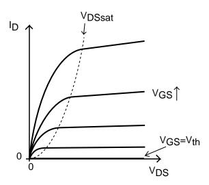
for  $L = 1 \ \mu m$ , increase of  $V_{DS}$  of 1 V past  $V_{DSsat}$  results in increase in  $I_D$  of 10%.
