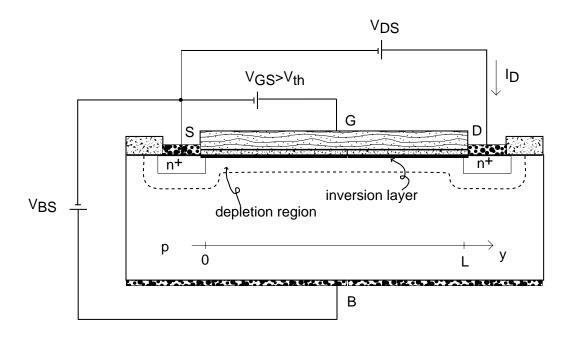
Body contact allows application of bias to body with respect to inversion layer,  $V_{BS}$ .
