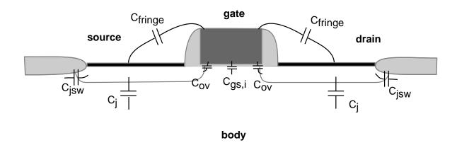
$C_{gs} \equiv \text{channel charge} + \text{overlap capacitance}, C_{ov}$  $C_{gd} \equiv \text{overlap capacitance}, C_{ov}$
