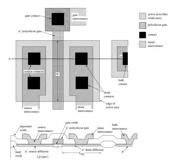
Body-to-source capacitance = source junction capacitance:
