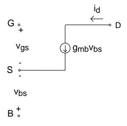
Complete MOSFET small-signal equivalent circuit model for low frequency:
