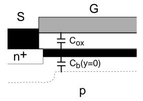
Handy rule: ratio of back transconductance to transconductance is equal to ratio of depletion capacitance at source to oxide capacitance.
