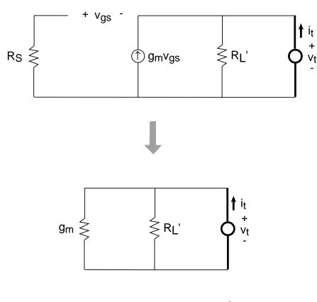
$$R_{Tdb} = \frac{1}{g_m} / / R_L' = \frac{R_L'}{1 + g_m R_L'}$$
