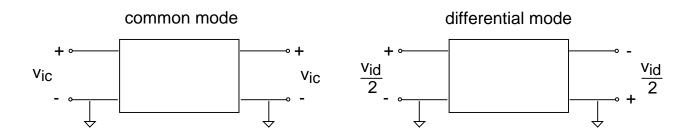
2. Exploit symmetry: break circuit into two "half circuits"
