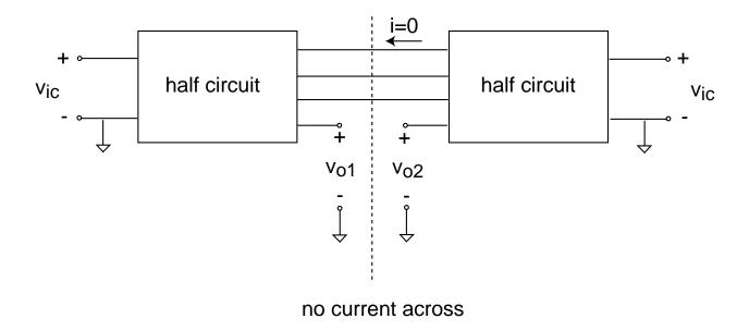
No current across wires connecting two half circuits  $\Rightarrow$  circuit identical to:
