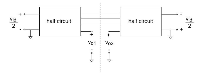
No voltage relative to ground along axis of symmetry  $\Rightarrow$  circuit identical to:
