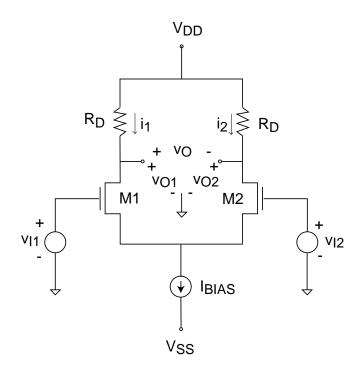
The higher  $r_{ob}$ , the smaller the change in  $I_{BIAS}$  in response to a common-mode signal  $\Rightarrow$  the smaller the change in  $v_{01}$  and  $v_{o2}$ .
