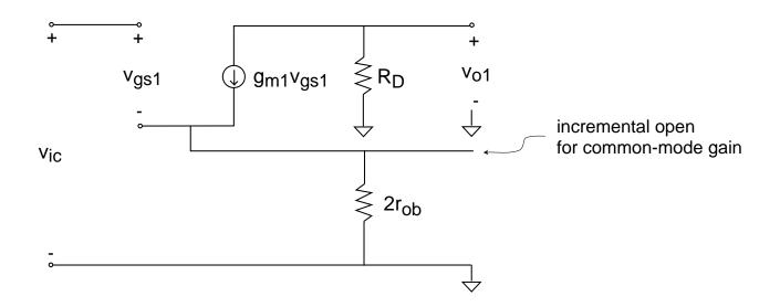
$$v_{o1} = -\frac{g_{m1}R_D}{1 + 2g_{m1}r_{ob}}v_{ic}$$
