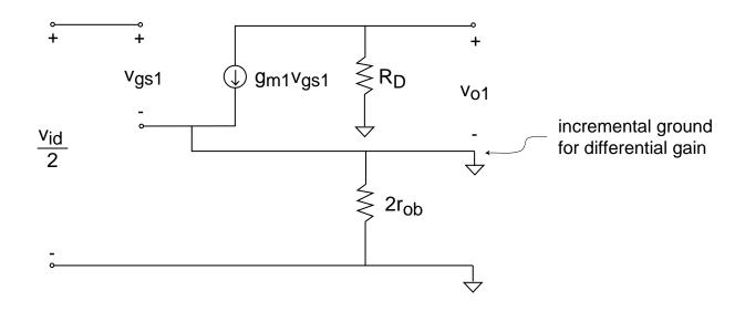
$$v_{o1} = -g_{m1}R_D \frac{v_{id}}{2}$$
