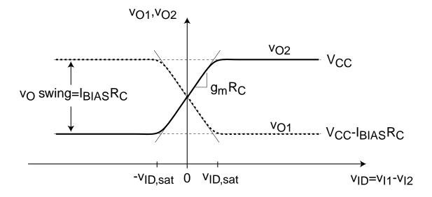
Differential input voltage to saturate amplifier:
