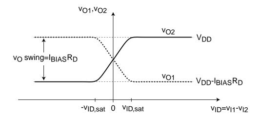
$v_{ID}$  that leads to amplifier saturation  $(v_{I1} \gg v_{I2})$ :
