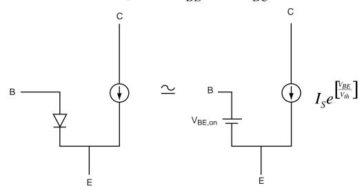
For today's technology:  $V_{BE,on} \approx 0.7 \ V. \ I_B$  depends on outside circuit.
