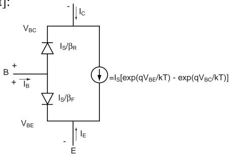
Three parameters in this model:  $I_S$ ,  $\beta_F$ , and  $\beta_R$ .
