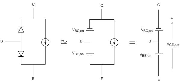
For today's technology:  $V_{CE,sat} \approx 0.1~V.~I_C$  and  $I_B$  depend on outside circuit.
