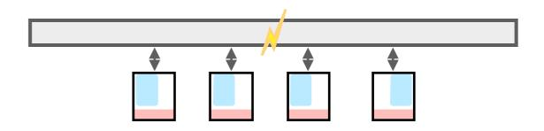
Circuit- or **packet-switching** lets multiple nodes share a network, even when there are many connections between nodes
