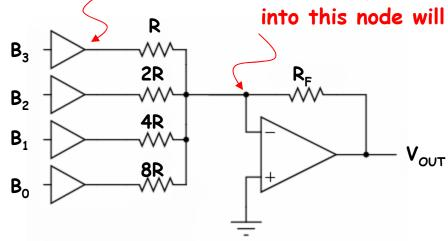
OKAY, this'll work, but the voltages produced by the drivers and various R's must be carefully matched in order to get equal steps.
