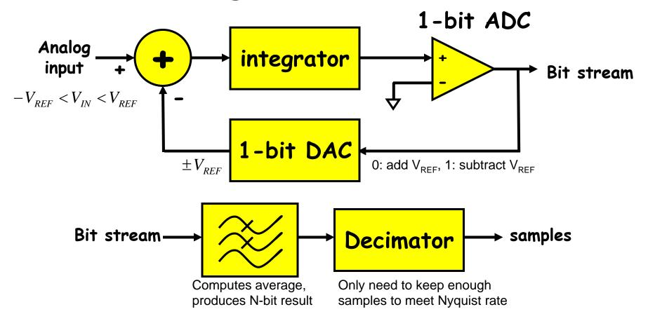
Average of bit stream  $(1=V_{REF}, 0=-V_{REF})$  gives voltage
