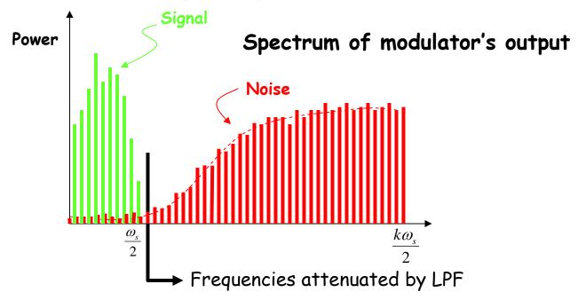
• Pushing noise power to higher frequencies means more noise is eliminated by LPF:  $N^{th}$  order  $\Sigma\Delta$  SNR = (3+N\*6)dB/octave
