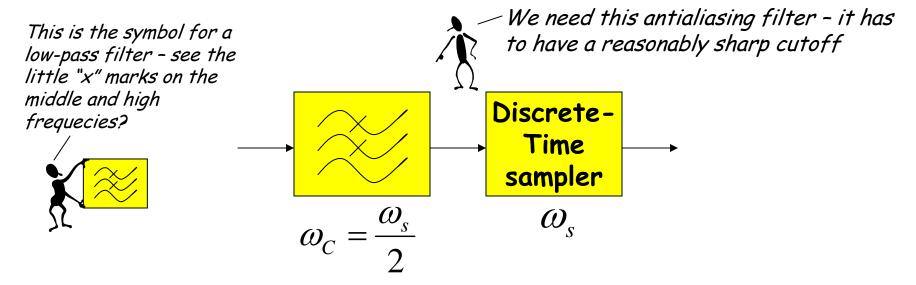
The frequency response of human ears essentially drops to zero above 20kHz. So the "Red Book" standard for CD Audio chose a 44.1kHz sampling rate, yielding a Nyquist frequency of 22.05kHz. The 2kHz of elbow room is needed because practical antialiasing filters have finite slope...
