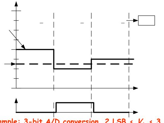
Example: 3-bit A/D conversion, 2 LSB  $< V_{in} < 3$  LSB
