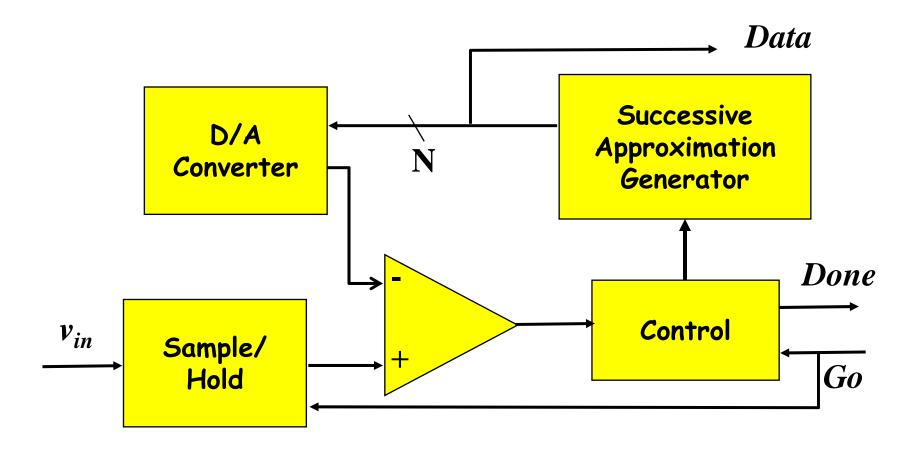
Serial conversion takes a time equal to  $N(t_{D/A} + t_{comp})$
