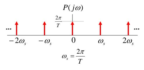
So, if  $\omega_m < \omega_s - \omega_m$ , we can recover the original waveform with a low-pass filter!
