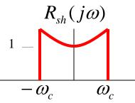
$$\omega_{M} < \omega_{c} < \omega_{s} - \omega_{M}$$
