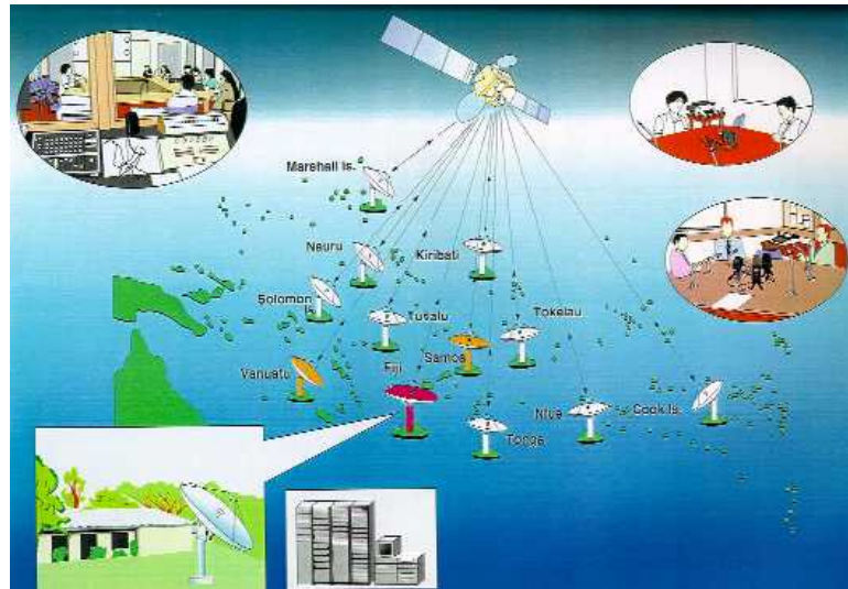
Figure 10-2: A satellite network. The “uplinks” from the ground stations to the satellite form a shared medium. (Picture from http://vidconf.net/ )
