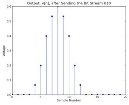
This plot shows the outputs of the input stream '010' and looking at sample 8, we see that the received voltage value for the transmitted current bit '1' is 0.6.
