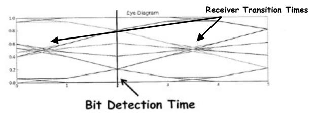
we can see that at the bit detection time, the received sample voltage can take on 6 different values. Remember, thus far we have not included any noise. We are looking at the noise free channel. The voltage value of the received sample is dependent on the previously transmitted bit, the current bit, and the next bit.
