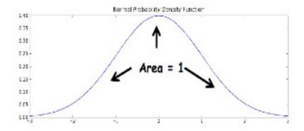
Let's begin by calculating the first term in our BER,  $P_{(000)1}$ . We look at the *noise free* + *noise* distribution and find that we have the noise distribution above centered around 0.0 and our error is the part of the Gaussian tail greater than  $0.5=V_{thresh}$ .
