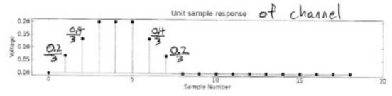
If we look at the output for an input stream of 3 Samples/bit, we see the following at the receiver:
