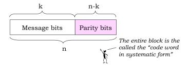
Figure 6-5: A code word in systematic form for a block code. Any linear code can be transformed into an equivalent systematic code.
