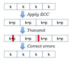
Figure 6-7: Dividing a long message into multiple SEC-protected blocks of k bits each, adding parity bits to each constituent block. The red vertical rectangles refer are bit errors.
