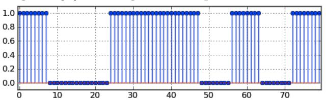
Example of distorted noise-free signal y[n] at receiver
