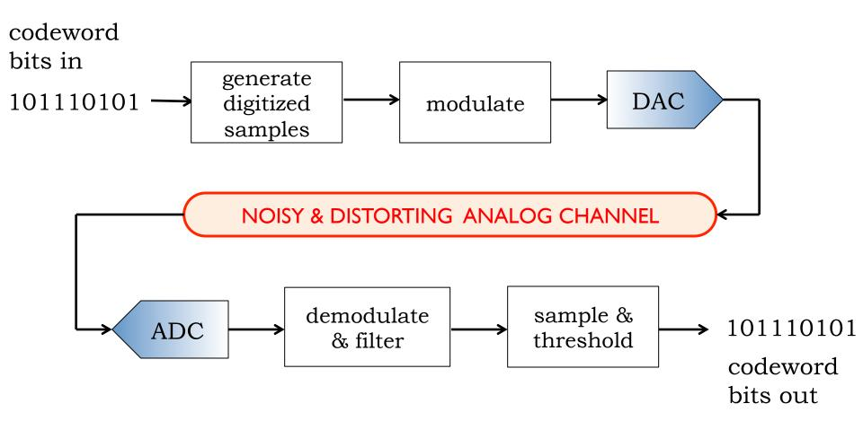
DAC: Digital-to-analog converter ADC: Analog-to-digital converter
