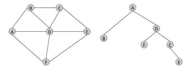
She discovers that the routing tree computed by Dijkstra's algorithm at node A looks like the picture on the **right, above**. Note that the exact order in which the nodes get added in Dijkstra's algorithm is not obvious from this picture.
