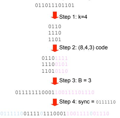
Sync pattern has five consecutive 1's. To prevent sync from appearing in message, "bit-stuff" 0's after any sequence of four 1's in the message. This step is easily reversed at receiver (just remove 0 after any sequence of four consecutive 1's in the message).
