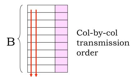
Problem: Bits from a particular codeword are transmitted sequentially, so a B-bit burst produces multi-bit errors.
