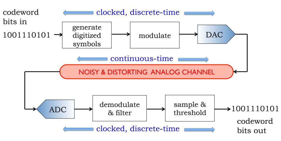
DAC: Digital-to-analog converter ADC: Analog-to-digital converter
