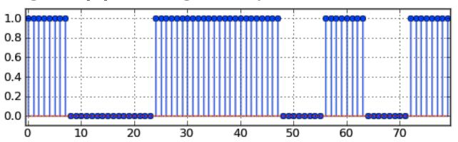
Distorted noise-free signal y[n] at receiver
