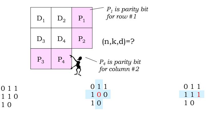
Parity for each row and column is correct ⇒ no errors
