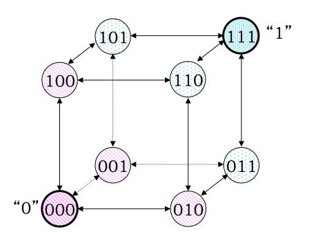
Code: A choice of 2<sup>k</sup> out of 2<sup>n</sup> nodes; a one-to-one mapping of all k-bit message strings to n-bit codewords.
