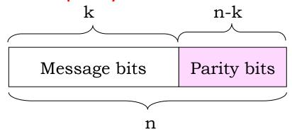
Every linear code can be represented by an equivalent systematic form --- ordering is not significant, direct inclusion of k message bits in n-bit codeword is.
