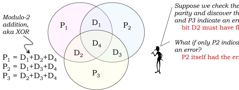
Suppose we check the parity and discover that P1 and P3 indicate an error? bit D2 must have flipped
