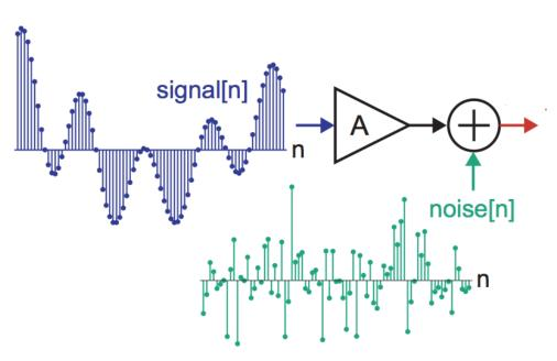
Changing the amplification factor (gain) A leads to different SNR values:
