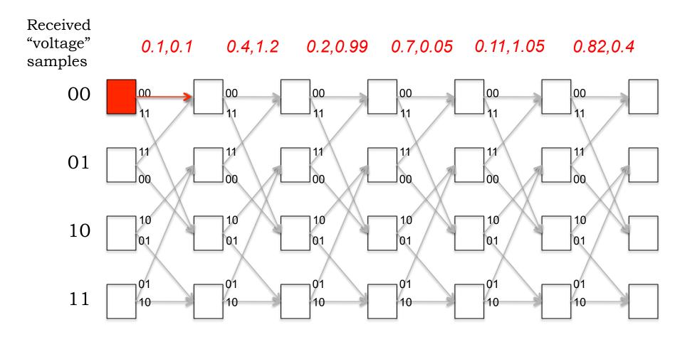
Given received "voltage" samples, find most-likely path through trellis, i.e., minimize "distance" between the received values and those produced along the trellis path.
