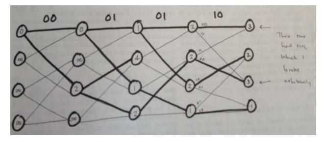
Having completed four iterations, let's look at the states. Which one was the transmitter most likely in at this point? State [11]: it has the smallest path metric.
