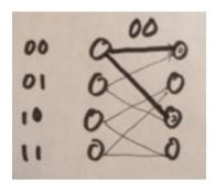
Notice that I am putting an error metric in the states. This indicates the error metric for the path that ends at that particular state in this iteration. You should immediately ask yourself: what happens if multiple paths end at the same state? This is a question I will answer shortly.
