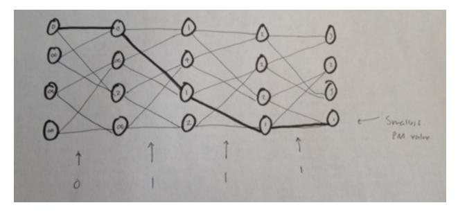
In this case we were able to correct the bit error. Without calculating the parity bits for that message, can you tell where the bit error came about in our received message? It happened between step 1 and 2. This is where the path metric for our chosen path increased from 0 to 1. (Note: this process worked because in this case we were able to decode the message correctly.)
