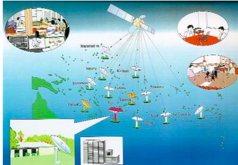
Figure 18-2: A satellite network. The “uplinks” from the ground stations to the satellite form a shared medium. (Picture from http://vidconf.net/ )
