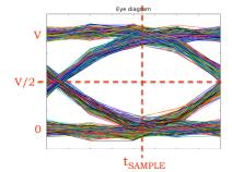
The good news: Our digital signaling scheme usually allows us to recover the original signal despite small amplitude errors introduced by inter-symbol interference and noise. An example of the digital abstraction doing its job!
