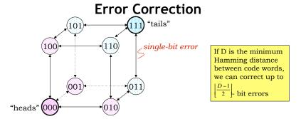
By increasing the Hamming distance between valid code words to 3, we guarantee that the sets of words produced by single-bit errors don't overlap. So if we detect an error, we can perform *error correction* since we can tell what the valid code was before the error happened.
