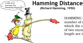
HAMMING DISTANCE: The number of digit positions in which the corresponding digits of two encodings of the same length are different
