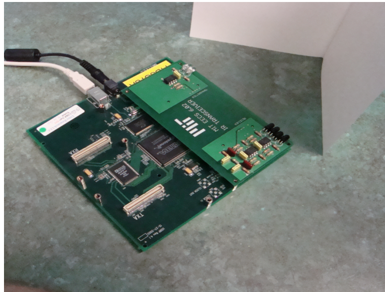
Figure 1-2: The experimental apparatus used in 6.02. The device uses infrared frequencies and includes both transmitter and receiver (transceiver).
