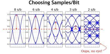
Given h[n], you can use the eye diagram to pick the number of samples transmitted for each bit (N):
