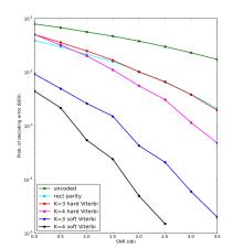
The graph shows how a rate  $\frac{1}{2}$ "rectangular" block code experimentally improves over using no coding at all, especially at higher SNRs (lower overall BER).
