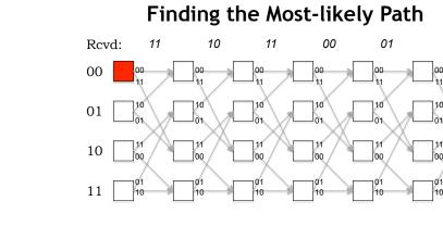
Given the received parity bits, the receiver must find the mostlikely sequence of transmitter states, i.e., the path through the trellis that minimizes the Hamming distance between the received parity bits and the parity bits the transmitter would have sent had it followed that state sequence.
