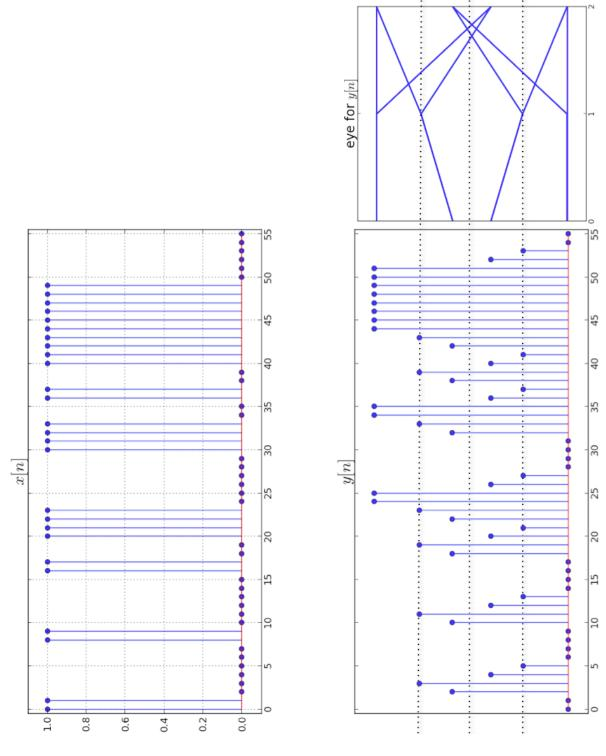
(C) (10 points) What are the possible voltages the receiver will see when it periodically samples y[n] at the widest part of the eye? Since the diagrams have no scale, you will need to compute the voltage values. To receive credit for this part you must show your work.
