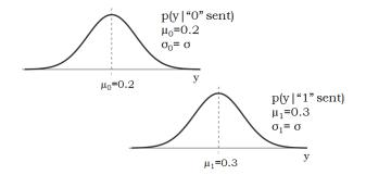
A. (2 points) Find the optimal receiver threshold if the prior probabilities of sending a "0" and "1" are equal, and the noise standard deviations on sending a "0" and "1" are also equal ( $\sigma_0 = \sigma_1$ ).
