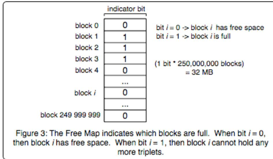
The Free Map uses 1 bit to represent each block on disk; therefore, a total of 32 MB is used to represent all 250,000,000 blocks. The pointers to the partitions take up negligible space in memory. The Free Map and the partition pointers are both written to disk during shutdown, and they are both read from disk during system startup.
