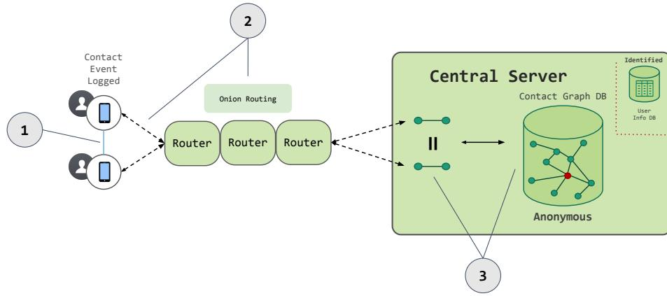
**Figure 3:** This figure illustrates the series of events when a user is involved in a contact event (Section 3.1): 1) the phones first identify the event, which they 2) communicate anonymously to the server using onion routing, after which 3) the server verifies the event and updates the contact graph database.
