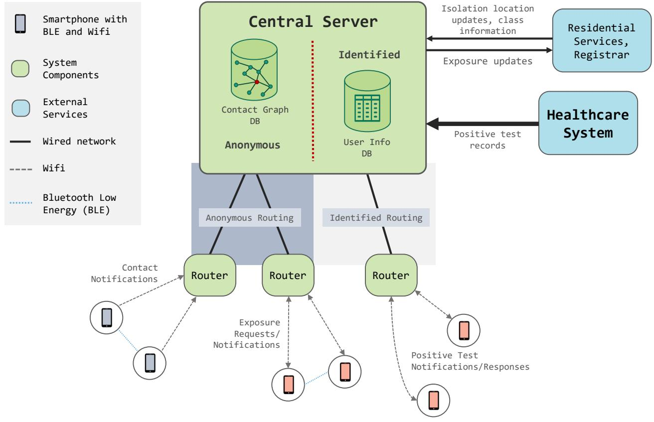
**Figure 1:** This System Diagram illustrates the three core components - the central server, the phones and the routers - as well as the three different communication protocols that the system uses - Bluetooth Low-Energy, anonymous onion routing and standard Ethernet and WiFi using TCP.
