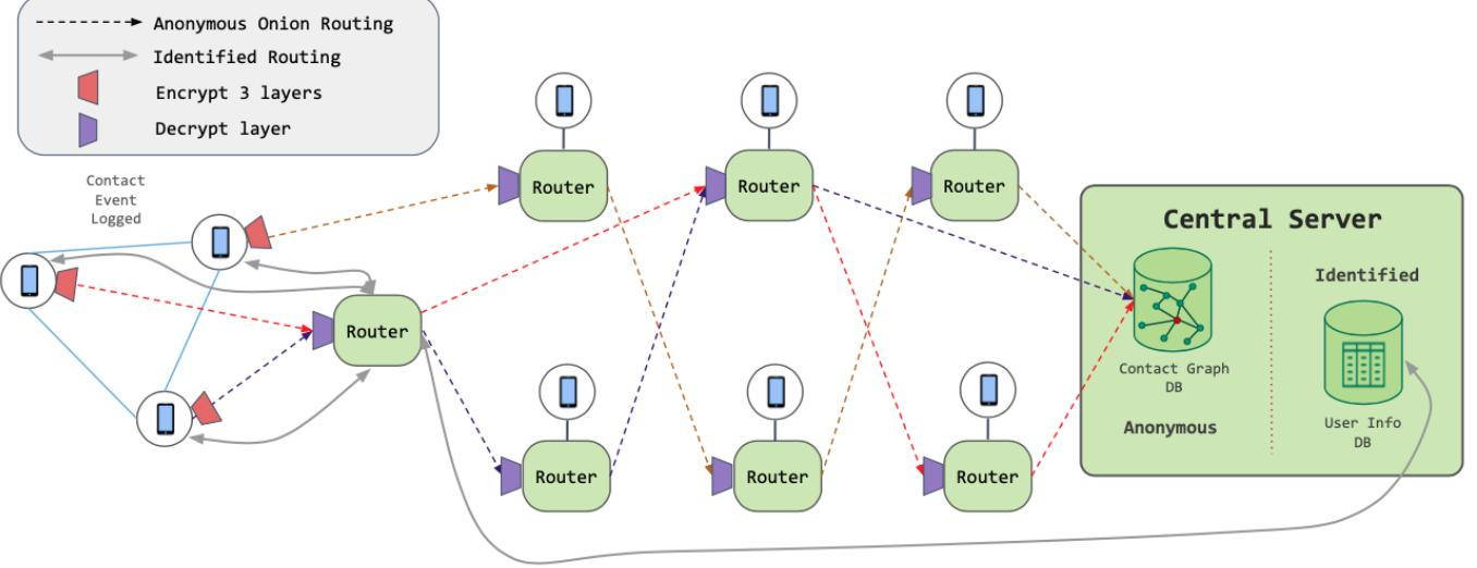
**Figure 2:** This figure illustrates how onion routing is used to hide the identity of the phone communicating with the central server. The message is encrypted three times over and each node (either the phone or router) knows only to decrypt the identify of the next node, thus by the time the message has reached the server, the server only knows the identity of the previous node.
