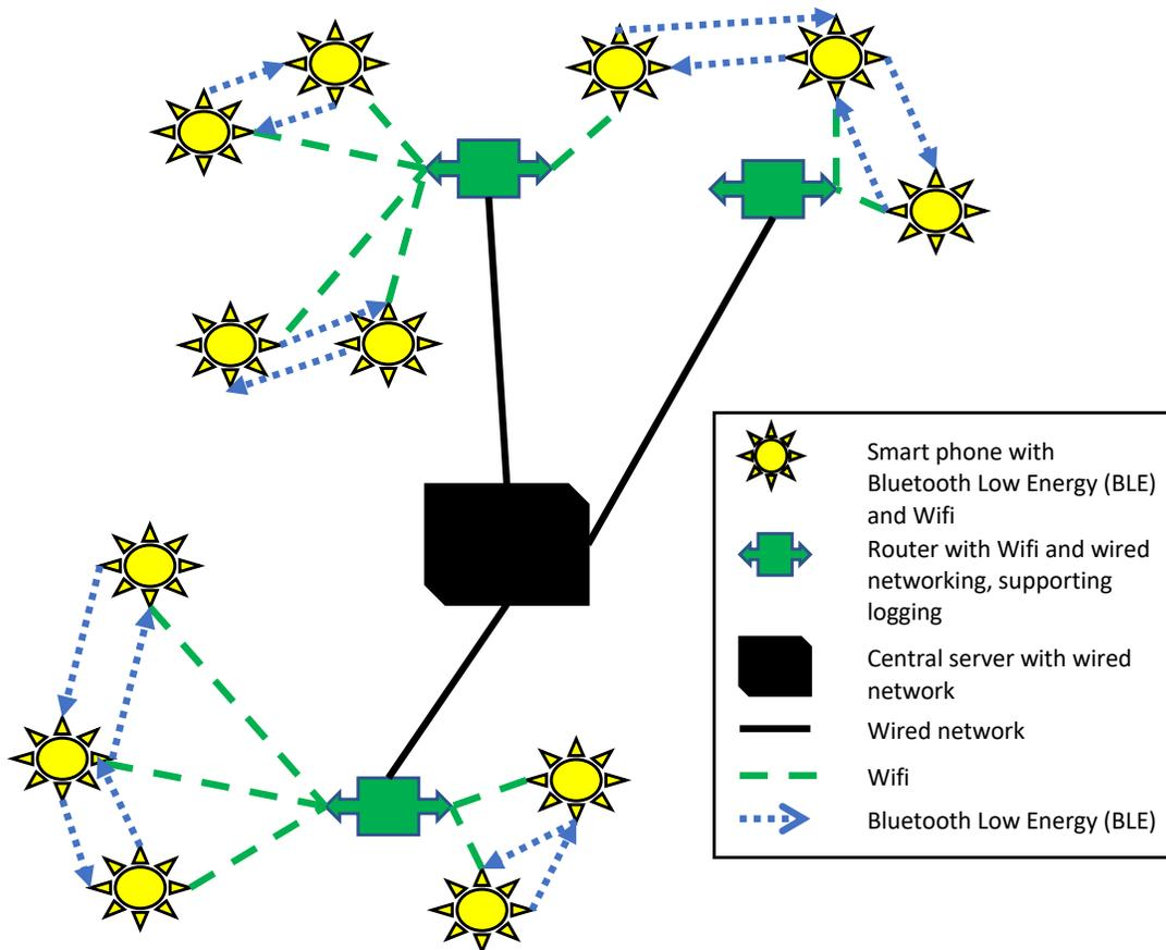
**Figure 1: A simplified system layout:** A central server is on the wired network. There is a collection of Wifi routers, both on the wired network and supporting Wifi devices. These are attached to walls, etc. and do not move. Then, there is a collection of smart phones, moving with their owners. Each smartphone supports both Bluetooth Low Energy (BLE), over which it broadcasts to nearby smart phones, and Wifi over which it can communicate with nearby routers.
