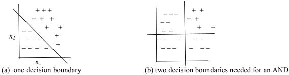
We can think of a step function net as defining a linear decision boundary, ax + by - c = 0. The sum of the weights of a step function neuron can represent the equation of the line:  $w_1x_1 + w_2x_2 - w_0 = 0$ . In example (a) above, to the left of the line can be represented by a 0 output; to the right a 1 output. Each decision line is represented by one neuron in the lowest layer of the net. Each class is represented by a neuron in the final layer,
