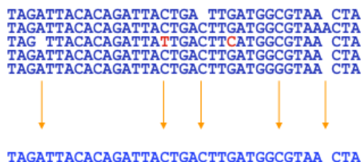
Figure 5.8: We derive the multiple alignment consensus sequence by weighted voting at each base
