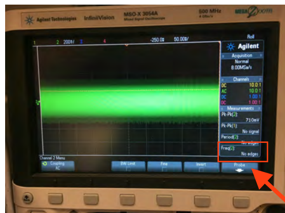
This is also noise. Notice that there is no discernible pattern, just a randomly fluctuating signal. The only thing we do know is that there is a lot of it (~700mV).
