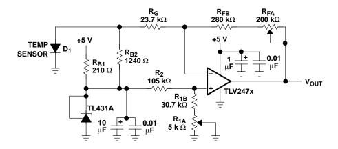
Figure 12-14. Final Analog Interface Circuit
