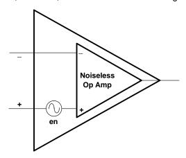
Figure 10-8. Equivalent Op Amp Circuit Noise Model
