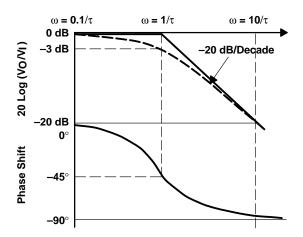
Figure 5–9. Bode Plot of Low-Pass Filter Transfer Function
