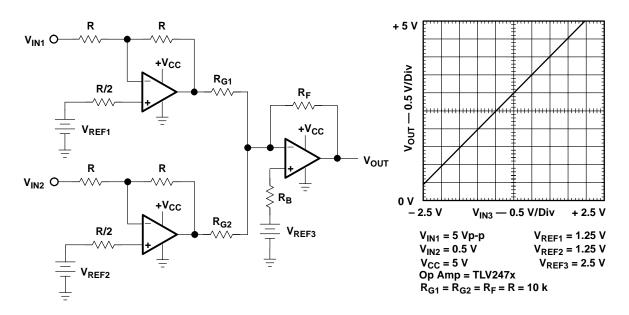
Figure A-26. Noninverting Summer with Buffers
