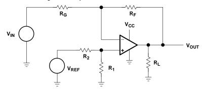
Figure 4–16. Schematic for Case 3:  $V_{OUT} = -mV_{IN} + b$
