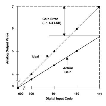
Figure 14-8. D/A Gain Error
