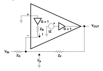
Figure 8-5. Inverting CFA
