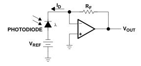
Figure 12–8. Photodiode Amplifier
