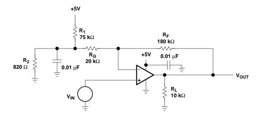
Figure 4-14. Case 2 Example Circuit
