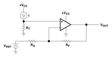
Figure 18–12. DAC Current Source to Actuator Interface Circuit
