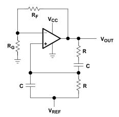
Figure 15–7. Wien Bridge Circuit Schematic
