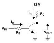
Figure 2–14. Saturated Transistor Circuit
