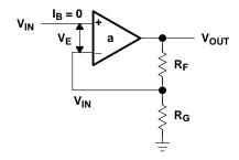
Figure 3-2. The Noninverting Op Amp
