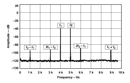
Figure 14–12. Intermodulation Distortion
