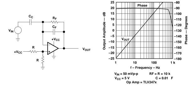
Figure A–36. Inverting Differentiator with Noise Filter
