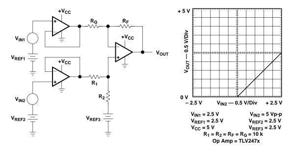
Figure A–18. Simplified High-Precision Differential Amplifier
