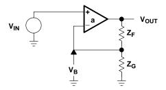
Figure 6-3. Noninverting Op Amp
