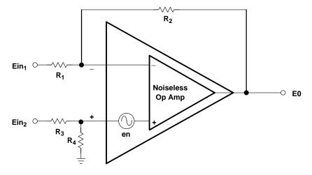
Figure 10-12. Differential Equivalent Op Amp Circuit Noise Model
