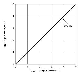
Figure 4-9. Transfer Curve for Noninverting Op Amp
