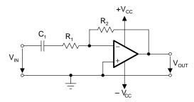
Figure 16-46. Dual-Supply Filter Circuit
