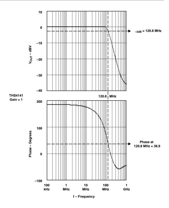
Figure 13–12. Differential Amplifier Closed-Loop Response
