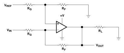
Figure 4-5. Inverting Op Amp
