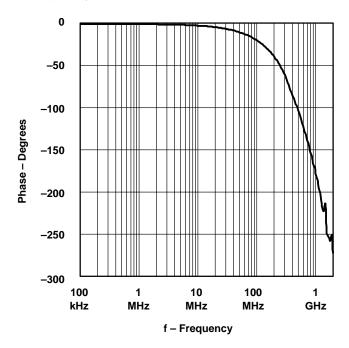
Figure 13-15. Phase vs Frequency for THS3201
