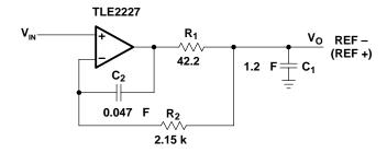
Figure 13-8. Voltage Reference Filter Circuit
