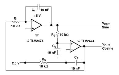
Figure 15–20. Quadrature Oscillator
