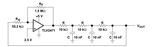
Figure 15-14. Phase Shift Oscillator (Single Op Amp)
