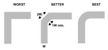
Figure 17-10. PCB Trace Corners
