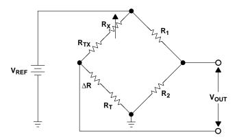
Figure 12-7. Wheatstone Bridge Circuit
