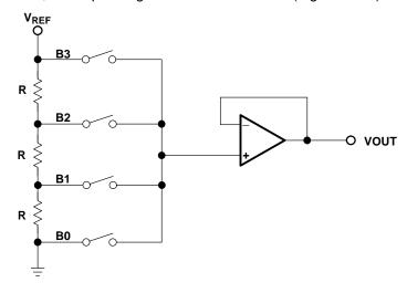
Figure 14-1. Resistor Ladder D/A Converter
