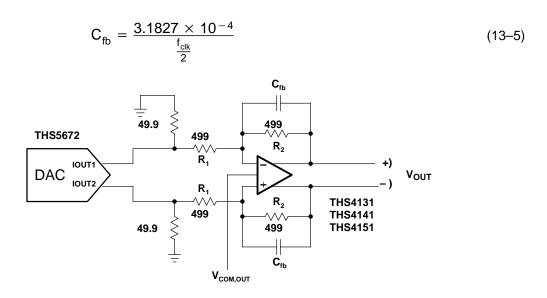
Figure 13-7. A Single-Pole Reconstruction Filter
