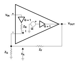
Figure 8-4. Noninverting CFA
