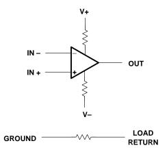
Figure 17-1. Op Amp Terminal Model
