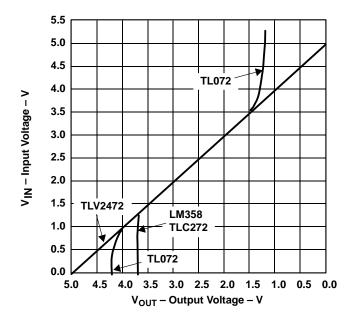
Figure 4–7. Transfer Curve for Inverting Op Amp With V<sub>CC</sub> Bias
