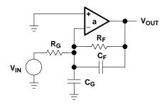
Figure 7–18. Compensated Attenuator Circuit
