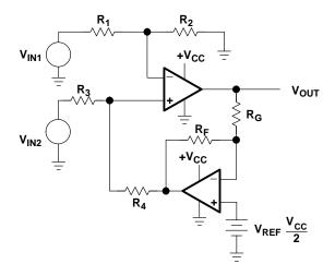
Figure A-19. Variable Gain Differential Amplifier
