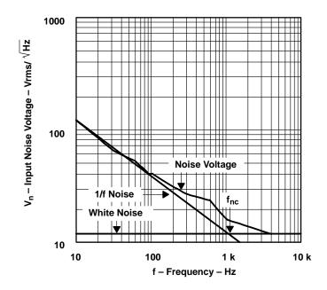
Figure 10-6. TLV2772 Op Amp Noise Characteristics
