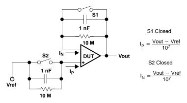
Figure 11–3. Test Circuit – I<sub>IB</sub>
