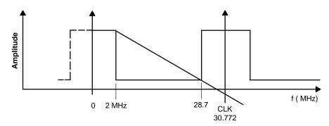
Figure 13-6. Reconstruction Filter Characteristics
