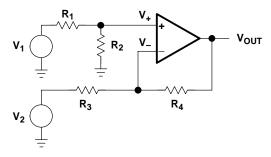
Figure 3-5. The Differential Amplifier
