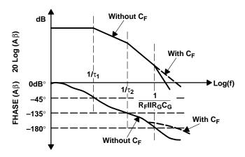
Figure 7-19. Compensated Attenuator Bode Plot
