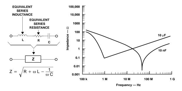
Figure 17–16. Capacitor Self Resonance
