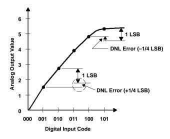
Figure 14-9. Differential Nonlinearity Error
