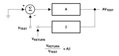
Figure 6-2. Feedback Loop Broken to Calculate Loop Gain
