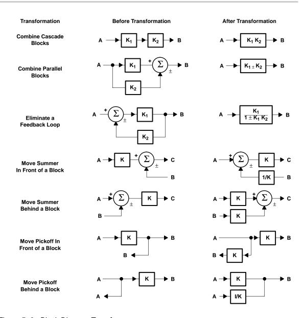
Figure 5-6. Block Diagram Transforms
