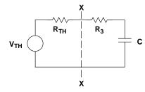
Figure 2–8. Thevenin's Equivalent Circuit for Figure 2–7
