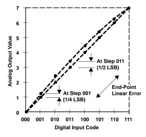
Figure 14–10. Integral Nonlinearity Error
