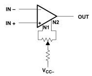
Figure 11-2. Offset Voltage Adjust
