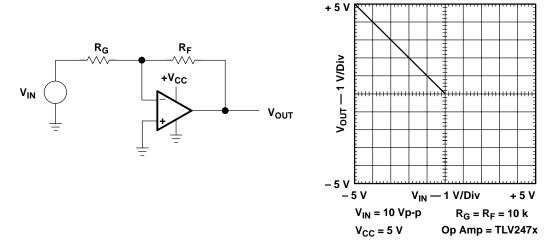
Figure A-4. Single-Supply Op Amp Circuit
