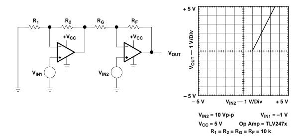
Figure A-15. High Input Impedance Differential Amplifier
