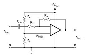
Figure 16–47. Single-Supply Filter Circuit
