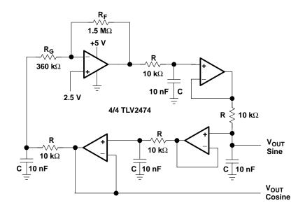
Figure 15-18. Bubba Oscillator
