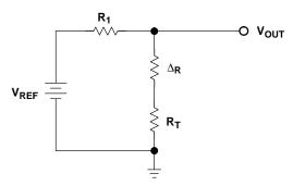
Figure 12-4. Voltage Divider Circuit for a Resistive Transducer
