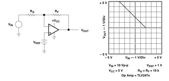
Figure A-5. Inverting Op Amp with Noninverting Positive Reference
