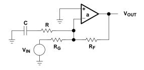
Figure 7-20. Lead-Lag Compensated Op Amp
