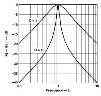
Figure 16–32. Gain Response of a Second-Order Band-Pass Filter
