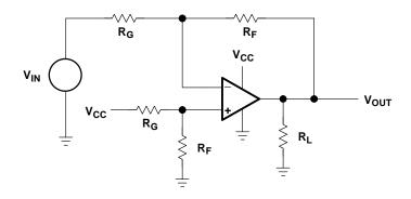
Figure 4-6. Inverting Op Amp With V<sub>CC</sub> Bias
