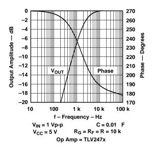
Figure A-22. Inverting AC Amplifier
