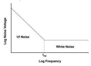
Figure 11–9. Typical Op amp Input Noise Spectrum
