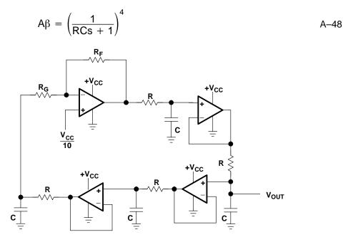
Figure A-43. Bubba Oscillator
