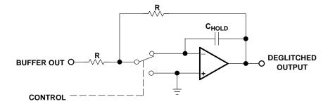
Figure 14-14. D/A Deglitch Circuit
