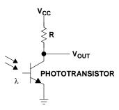
Figure 12-9. Phototransistor Amplifier
