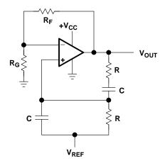
Figure A-37. Basic Wien Bridge Oscillator
