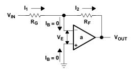
Figure 3–3. The Inverting Op Amp
