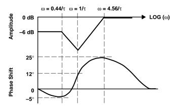
Figure 5-12. Combined Pole Zero Plot of Band Reject Filter
