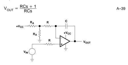
Figure A-34. Noninverting Integrator Approximation
