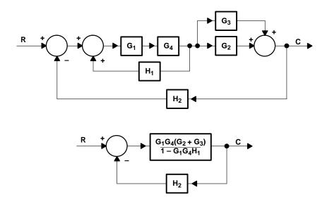
Figure 5-5. Multiloop Feedback System
