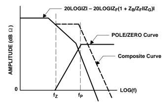
Figure 8–9. Bode Plot with C<sub>F</sub>
