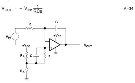
Figure A-29. Inverting Integrator with Drift Compensation
