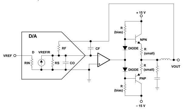
Figure 14–16. D/A Output Current Booster
