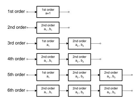
Figure 16–11. Cascading Filter Stages for Higher-Order Filters
