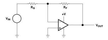
Figure 4-4. Single-Supply Op Amp Circuit
