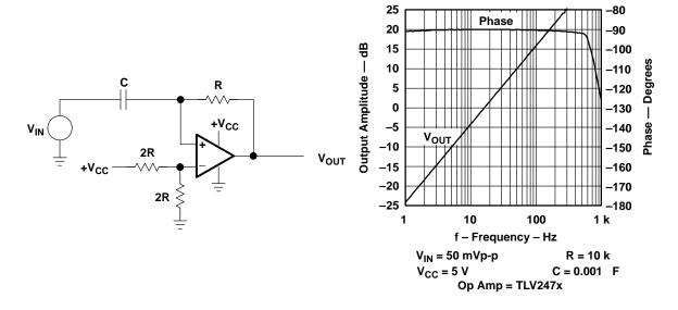
Figure A–35. Inverting Differentiator
