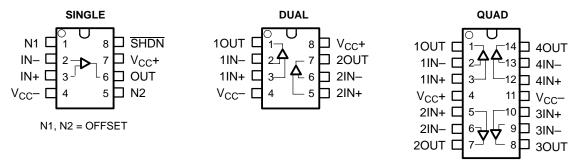
Figure 17–17. Common Op Amp Pinouts
