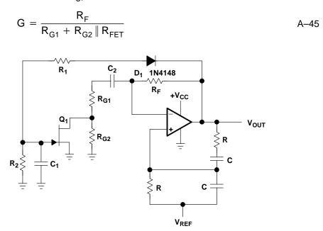
Figure A-39. Wien Bridge Oscillator with AGC
