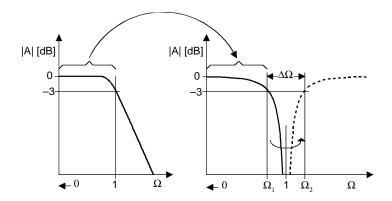
Figure 16-36. Low-Pass to Band-Rejection Transition
