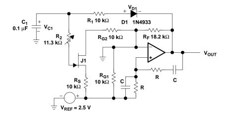
Figure 15-12. Wien Bridge Oscillator with AGC
