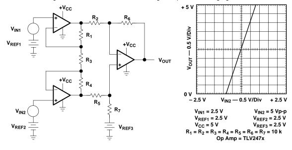
Figure A-17. High-Precision Differential Amplifier
