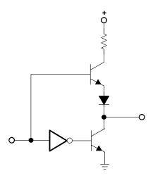
Figure 17-15. Logic Gate Output Structure
