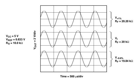
Figure 15-9. Wien Bridge Output Waveforms
