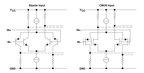
Figure 18-4. Input Circuit of an RRI Op Amp
