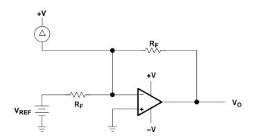
Figure 18–13. DAC Current Sink to Actuator Interface Circuit
