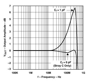
Figure 17-12. Effect of 1-pF Capacitance on Op Amp Inverting Input
