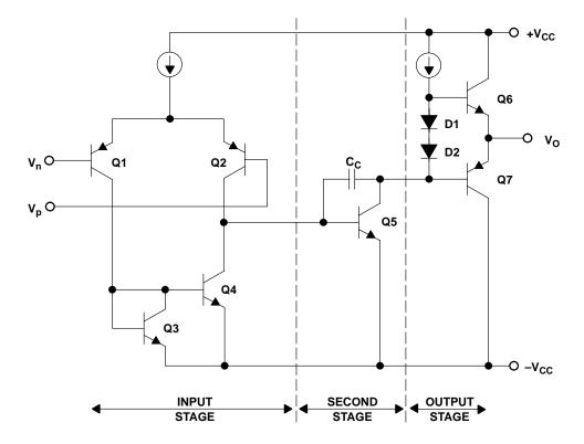
Figure 11-8. Figure 7. Simplified Op Amp Schematic
