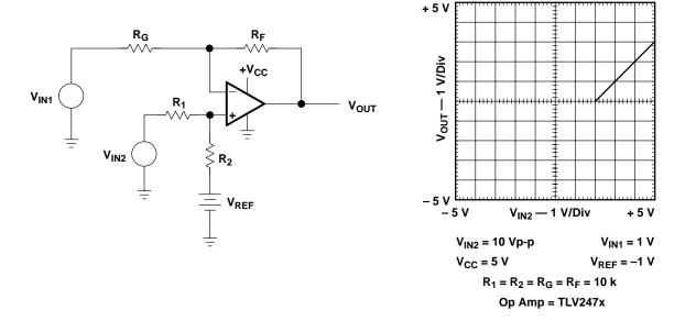
Figure A-14. Differential Amplifier with Bias Correction
