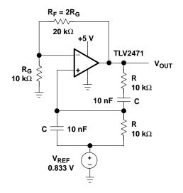
Figure 15-8. Final Wien Bridge Oscillator Circuit
