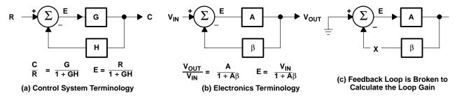
Figure 5-7. Comparison of Control and Electronic Canonical Feedback Systems
