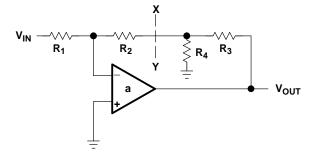
Figure 3–7. T Network in Feedback Loop
