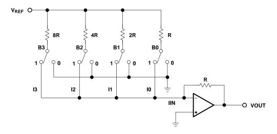
Figure 14-2. Binary Weighted D/A Converter
