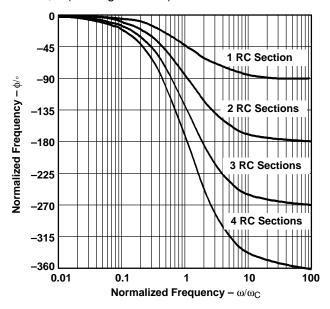
Figure 15-2. Phase Plot of RC Sections
