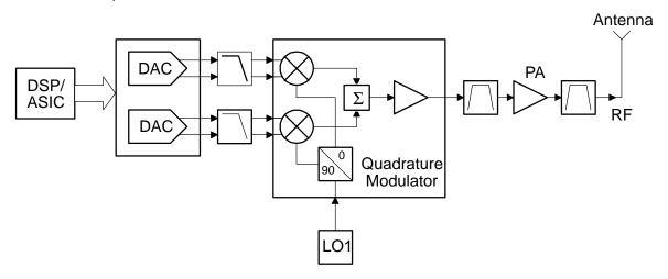
Figure 13-3. Basic W-CDMA Cellular Base Station Transmitter Block
