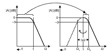
Figure 16-31. Low-Pass to Band-Pass Transition
