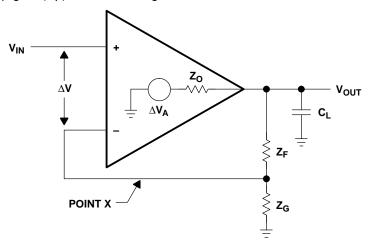
Figure 7-8. Capacitively-Loaded Op Amp
