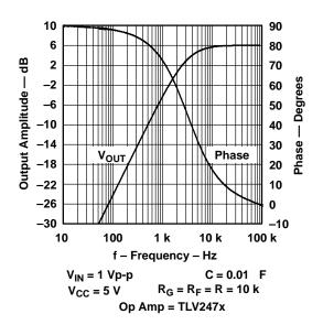
Figure A–23. Noninverting AC Amplifier
