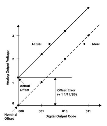
Figure 14-7. D/A Offset Error
