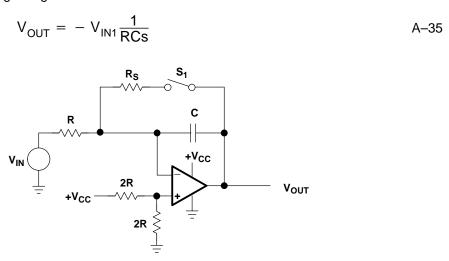
Figure A-30. Inverting Integrator with Mechanical Reset
