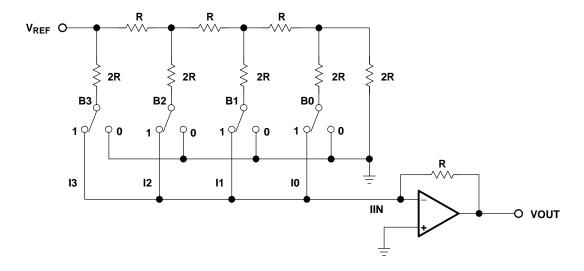
Figure 14–4. R/2R D/A Converter
