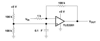
Figure 10–16. Improved TLC2201 Op Amp Circuit
