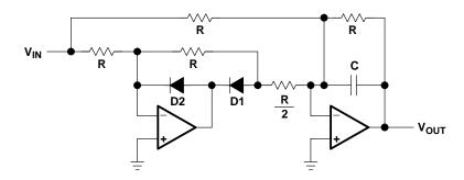
Figure 12-11. Active Full-Wave Rectifier and Filter
