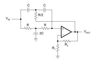
Figure 16-38. Active Twin-T Filter
