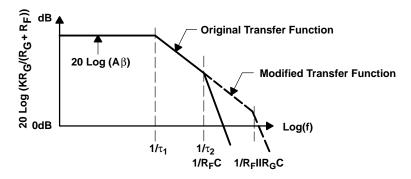
Figure 7–14. Lead-Compensation Bode Plot
