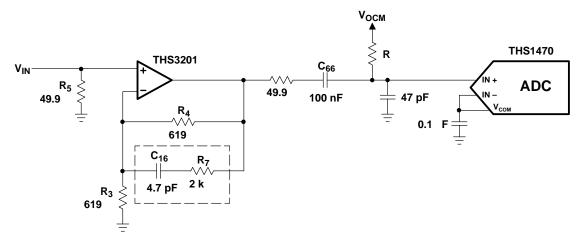
Figure 13-13. ADC Single-Ended Input Drive Circuit
