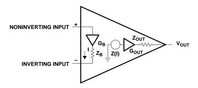
Figure 8-1. Current-Feedback Amplifier Model
