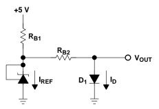
Figure 12-12. Reference and Transducer Bias Circuit
