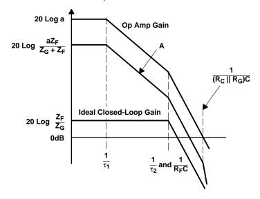
Figure 7-15. Inverting Op Amp With Lead Compensation
