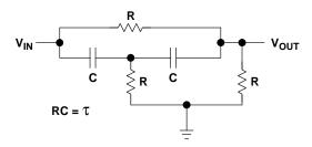
Figure 5–10. Band Reject Filter
