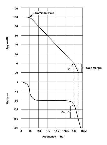
Figure 11–11. Voltage Amplification and Phase Shift vs. Frequency
