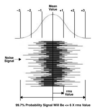
Figure 10–1. Gaussian Distribution of Noise Energy
