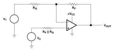
Figure 18–2. Noninverting Op Amp
