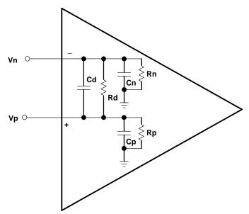
Figure 11-5. Input Parasitic Elements
