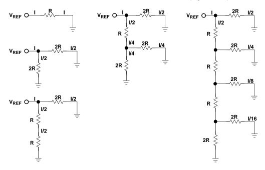
Figure 14–3. R/2R Resistor Array
