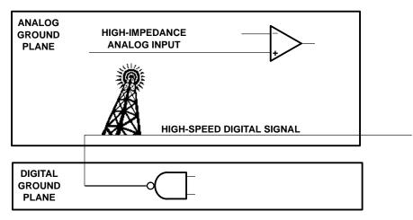
Figure 17-4. Broadcasting From PCB Traces
