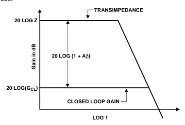
Figure 9-4. CFA Gain vs Frequency
