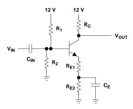
Figure 2–15. Transistor Amplifier
