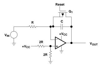
Figure A-31. Inverting Integrator with Electronic Reset
