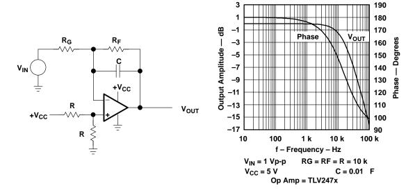
Figure A-32. Inverting Integrator with Resistive Reset
