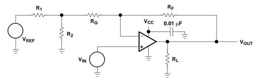
Figure 4–13. Schematic for Case 2:  $V_{OUT} = +mV_{IN-b}$
