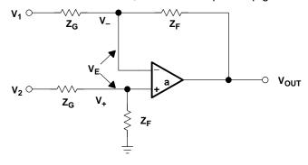
Figure 6–7. Differential Amplifier Circuit
