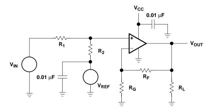
Figure 4–10. Schematic for Case 1:  $V_{OUT} = +mV_{IN} + b$
