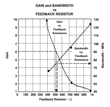
Figure 8–7. Plot of CFA R<sub>F</sub>, G, and BW
