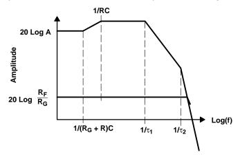
Figure 7–22. Closed-Loop Plot of Lead-Lag Compensated Op Amp
