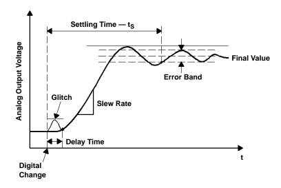
Figure 14-13. D/A Settling Time
