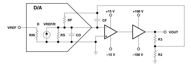
Figure 14-18. Correct Method of Increasing Voltage Range
