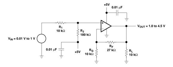
Figure 4-11. Case 1 Example Circuit
