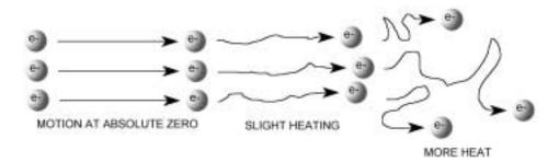
Figure 10-3. Thermal Noise
