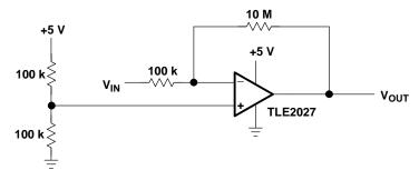
Figure 10-13. Split Supply Op Amp Circuit
