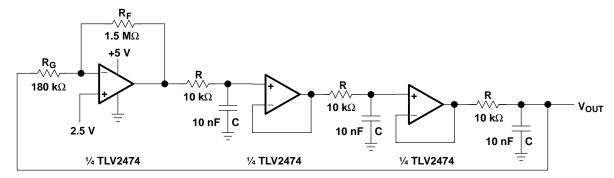
Figure 15–16. Phase Shift Oscillator, Buffered
