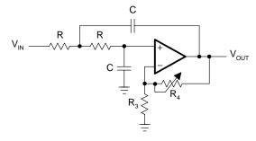
Figure 16–18. Adjustable Second-Order Low-Pass Filter
