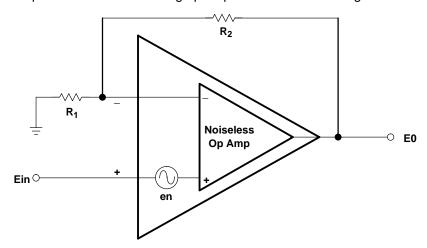
Figure 10–11. Noninverting Equivalent Op Amp Circuit Noise Model
