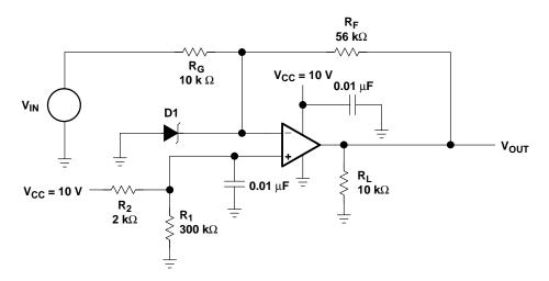
Figure 4-17. Case 3 Example Circuit
