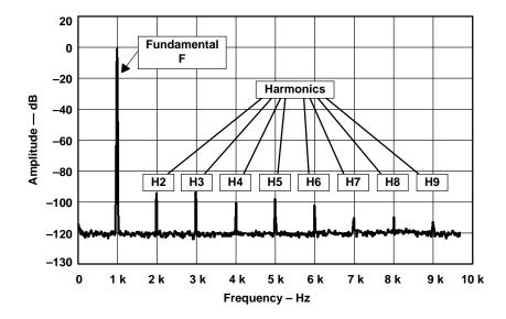
Figure 14-6. Total Harmonic Distortion
