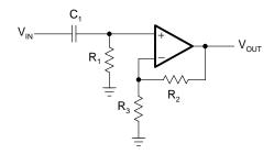
Figure 16–25. First-Order Noninverting High-Pass Filter
