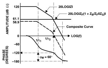
Figure 8-6. Bode Plot of Stability Equation
