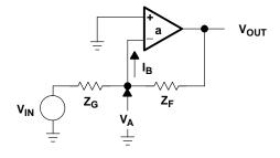
Figure 6-5. Inverting Op Amp
