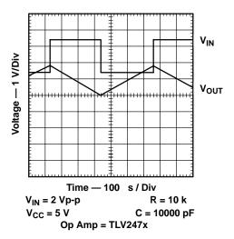
Figure A–27. Inverting Integrator
