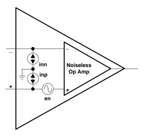
Figure 10–7. Op Amp Circuit Noise Model
