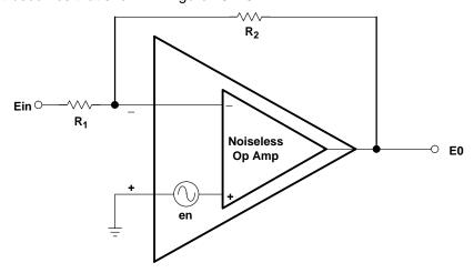
Figure 10-10. Inverting Equivalent Op Amp Circuit Noise Model
