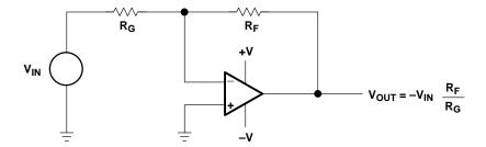
Figure 4–1. Split-Supply Op Amp Circuit
