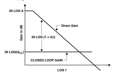
Figure 9–3. VFA Gain versus Frequency
