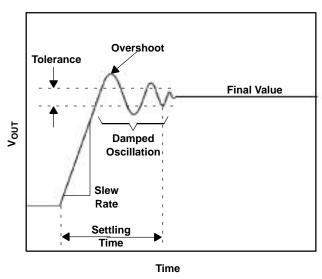
Figure 11–12. Settling Time
