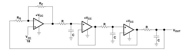
Figure A-42. Buffered Phase Shift Oscillator
