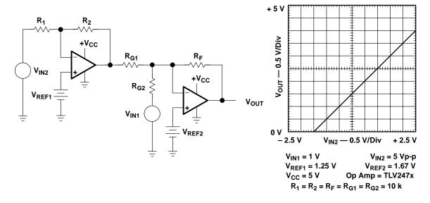
Figure A–16. High Common-Mode Range Differential Amplifier
