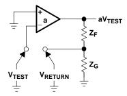
Figure 6-4. Open Loop Noninverting Op Amp
