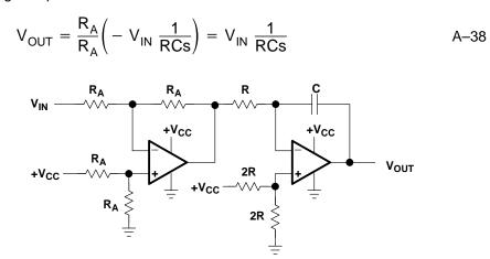
Figure A-33. Noninverting Integrator with Inverting Buffer
