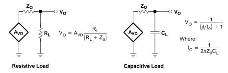
Figure 11-6. Effect of Output Impedance
