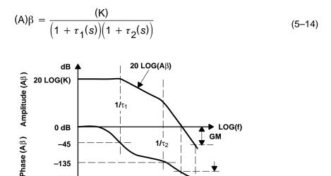
Figure 5–15. Magnitude and Phase Plot of Equation 5–14
