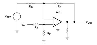
Figure 4-8. Noninverting Op Amp
