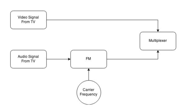
Goal: Convert signals from TV other device into a format for transmission
