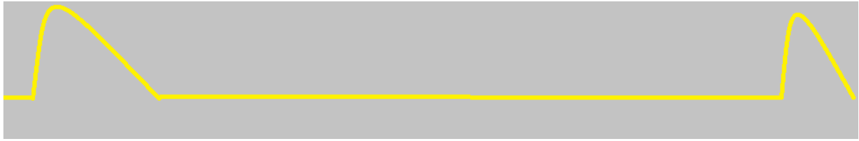
Figure 8- Mockup of the output of the peak detector. The received sine wave charges the capacitor and it then discharges through the resistor.
