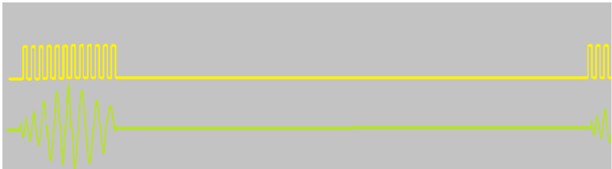
Figure 5- Figure 5 shows a mockup of the scope shot where the yellow trace represents the signal outputted from the transmitter circuit and the green represents the signal outputted by the ultrasound receiver. The yellow output has a peak to peak voltage of 5V while the green trace's peak to peak is ~50mV.
