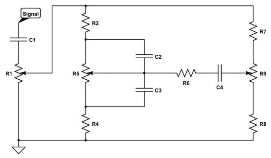
The tone control part of the circuit is first put into the circuit via C1 and R1. This acts as the gain control. The signal is then passed to a Baxendall tone control network. R5 is used to control the bass, and R9 is used to control treble. R1 should be a logarithmic type potentiometer. R5 and R9 should be linear type potentiometers. This will help the performer to easily control the tone control.
