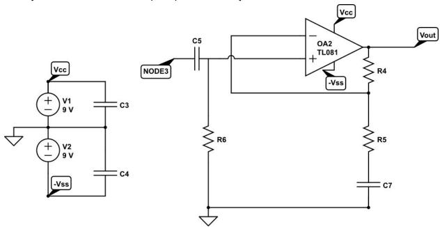
The preamplifier is an op amp in a non-inverting amplifier configuration. The gain of it is set by R4 and R5. These two values are calculated to give an output of around ~1V RMS line signal. C5 and R6 couple the signal to ground. R6 is set to an extremely high value of around 3-10 Mohm to get a high input impedance to the amplifier. Since C5 and R6 act as a high pass filter, C5 is selected to set the cutoff frequency to be below the lowest note of the violin.
