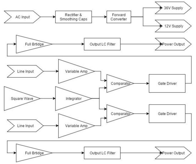
The amplifier stage of this project will be implemented as a class D amplifier. Our goal will be to make it capable of outputting at least 100w of power with minimal distortion between the frequencies created by a violin. Other target features will include AC input, a flat frequency response, line-level input, and volume control. The system will be implemented as follows:
