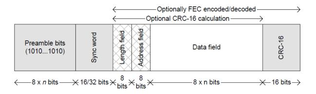
The preamble bits and sync word are used by the receiver for synchronization. For this problem, you will only be concerned with the three blocks of data consisting of the Length Field, Address Field and Data Field. FEC, forward error correction, is a technique that allows a receiver to correct errors in a received packet by convolving the data and sending the parity bits. More on FEC in Lpset #7.
