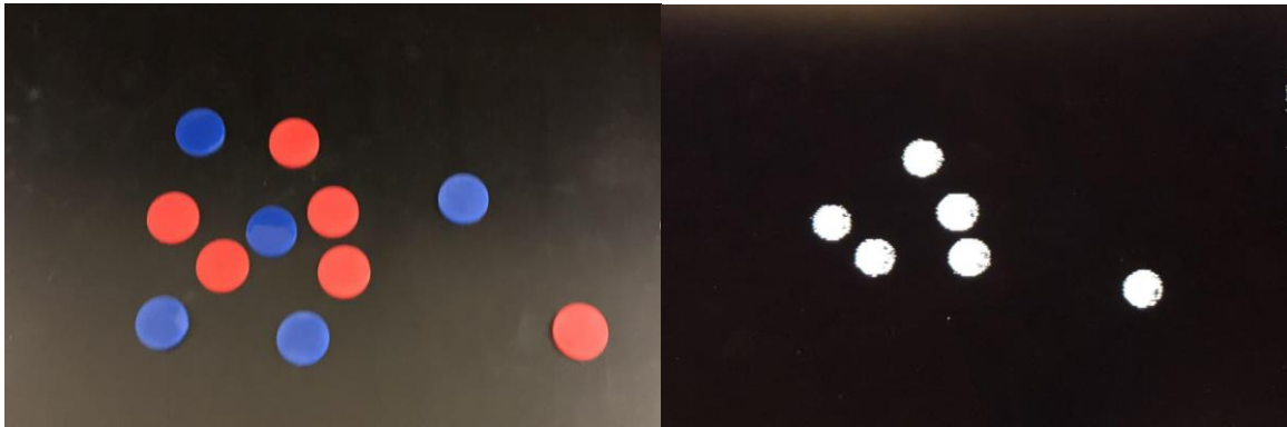
An example image of the HSV thresholding. The binarized mask only includes the red checkers.
