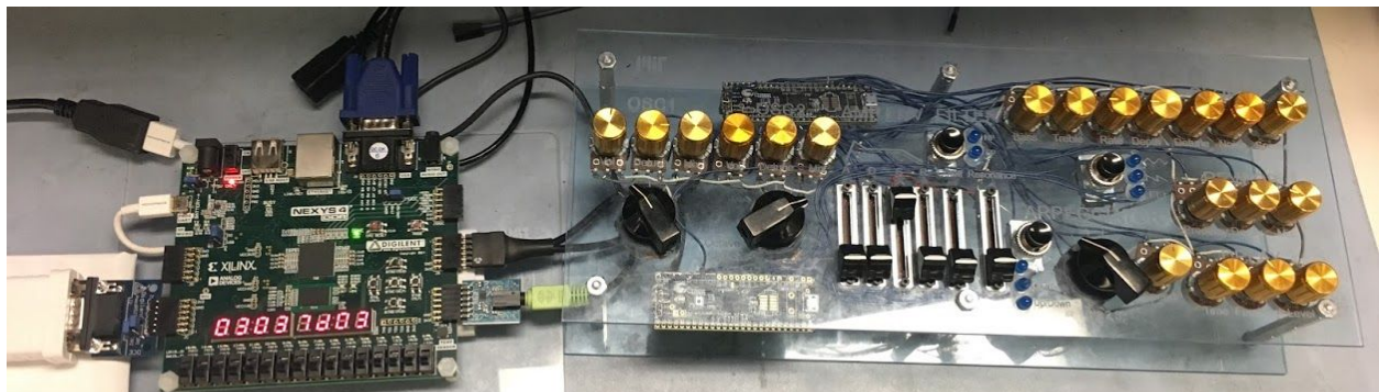
Figure 9: Photo of control panel, Nexys4 FPGA, and PMODs
