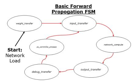
The high level graphical description of the state machine can be seen in figure above. Specifically, the mechanism for performing forward propagation as follows.
