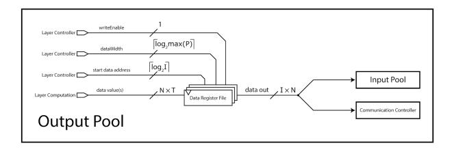
The Output Pool serves as the buffer for Layer Computation outputs. As opposed to the Input Pool, which modifies the entire register file on a write operation, the output pool uses the data start address and data width values from the Layer Controller to determine which registers to write to when writeEnable is asserted. The data from this register file is forwarded to the Input Pool and the Communication Controller for appropriate further processing.
