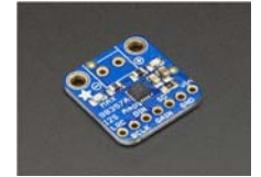
MAX98357A-based board from Adafruit: 3W Class D audio amp i2s input
