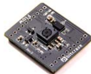
Board with combined PMW3901 and VL53L0X (optical flow and distance)
