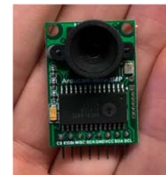
Front chip is a video frame buffer
