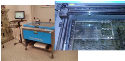
Laser cutter – PSL6.75 with 75W laser Part size: 32" x 18" x 9" Cut by "printing"
