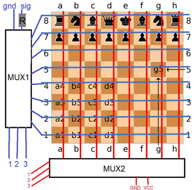
A submodule will wait for a get\_pos signal and then run through 64 permutations activating and deactivating vertical and horizontal wires. The corresponding high and low signal will be used by another module that will generate a 64-bit long number that shows which squares of the chess board have figures on them.
