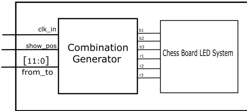
One input to this module is the show\_pos signal to start displaying the needed movement of the figures. The from\_to signal is a 12-bit long signal. First 6 bits are designated to signal the coordinate of the “from” LED while the last 6 bits are to signal the “to” LED. The two LED’s will turn on and off alternatively until the player moves the figure.
