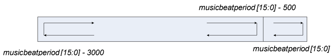
Figure 17: Note extend works by reversing the playback once the address reaches musicbeatperiod[15:0] . Playback will reverse again after reaching musicbeatperiod[15:0] - 3000 . After reaching musicbeatperiod[15:0] - 500 , playback will reverse again. Thus, playback is contained within musicbeatperiod[15:0] - 3000 and musicbeatperiod[15:0] - 500 .
