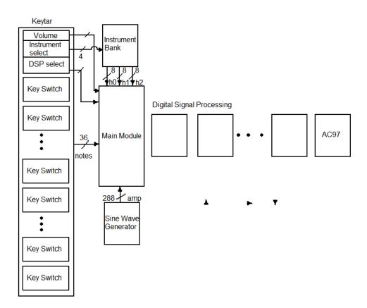
Figure 1: Block diagram for the keytar handler
