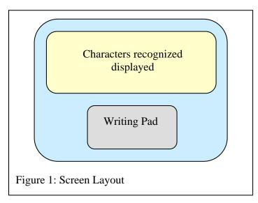
The project will implement characters by storing the direction the mouse moves as it traces out a character. These directions are matched against a memory array that details the motion the mouse is expected to make when tracing out valid characters. Once a match is found between the input and the table, the character is displayed to the screen.
