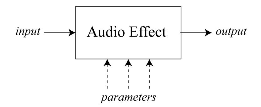
The signal transformation that occurs within a given audio effects block are determined by the parameter signals/constants fed into that module.
