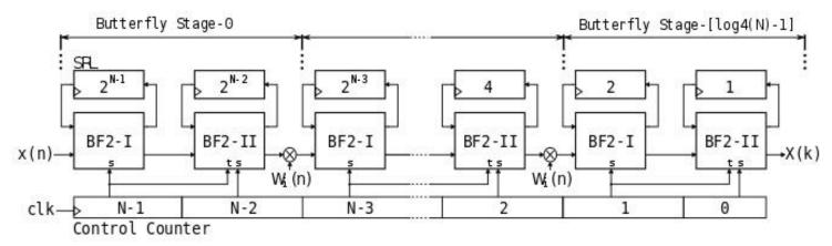
Radix 2<sup>2</sup> Single Delay Feedback architecture.
