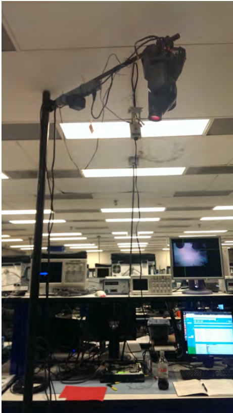
Figures 12 and 13: On the left, Figure 12 shows the test rig from far away. The light is attached to the sidearm which is clamped to the vertical pipe. There is a power strip attached to the sidearm which powered the light and the camera. On the right, Figure 13 shows the test rig from below. The relationship between the camera and the light's positions in the xy plane can be seen more easily
