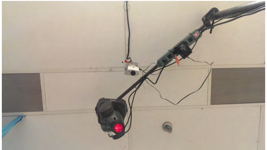
Figures 12 and 13: On the left, Figure 12 shows the test rig from far away. The light is attached to the sidearm which is clamped to the vertical pipe. There is a power strip attached to the sidearm which powered the light and the camera. On the right, Figure 13 shows the test rig from below. The relationship between the camera and the light's positions in the xy plane can be seen more easily
