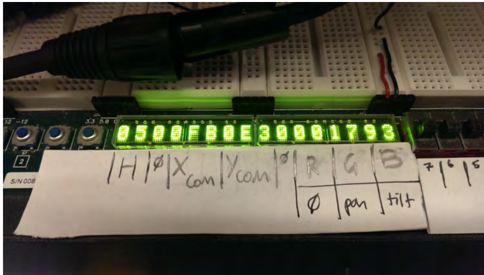
Figure 11: The 16 hex displays working. The labels describe what each hex display location represents. From left to right, it displays the hue, then nothing, then x com and y com , then nothing, then the pan and tilt bytes. Previously it displayed RGB values as shown by the label
