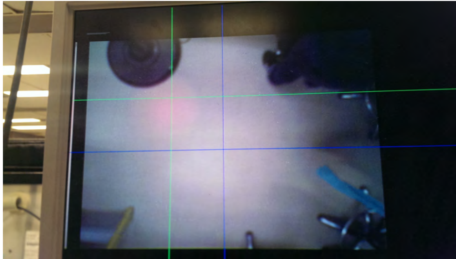
Figure 12: A photos of the display in cursor mode. The red light can be seen faintly at the location of the green cursors' intersection.
