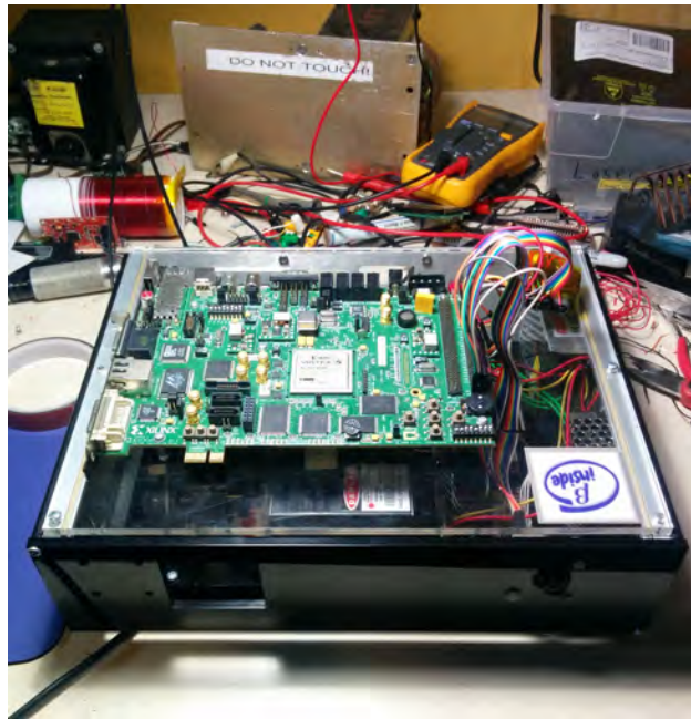
Figure 14: The housing for the laser and camera system, FPGA mounted on top.
