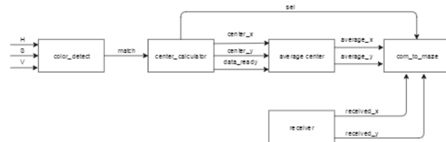
Figure 6 Detailed Block Diagram of Object-Recognition and Tracking Subsystem
